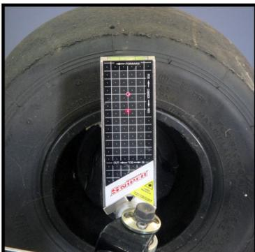
The Inox can be checked for accuracy by recording your settings and then swapping the units left to right and you should see the same settings (toe in/out will be back to front).
