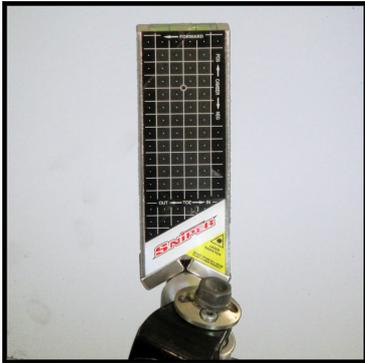
The Inox uses a magnetized Vee Block to locate onto the spindles, therefore the spindles must be clean and free from rust, especially make sure that no metallic debris is stuck to the Vee.
