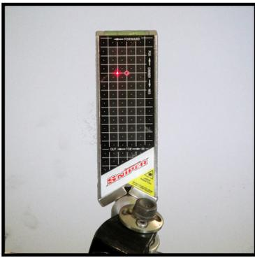
You are now ready to begin adjustment of toe and camber. The laser dot in the center of the grid is the beam shining out at the opposing unit. Readings are then taken from the unit opposite to the stub axle being adjusted.
