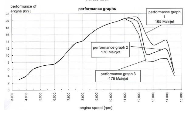
As you can see from the graph above, correct jetting has a direct impact upon performance. In the example the correct jet for the day was a 165.
