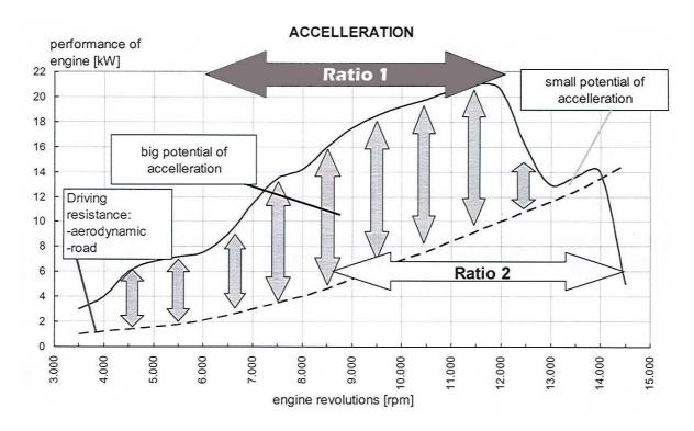
The top curve in the diagram above represents the power curve of the engine under load. When selecting 'Ratio 1' which is the lower of the two rear sprockets the engine performs peak efficiency, when selecting 'Ratio 2' the engine spends too much time in the 12,000 to 14,000 rev range when less horsepower is developed.
