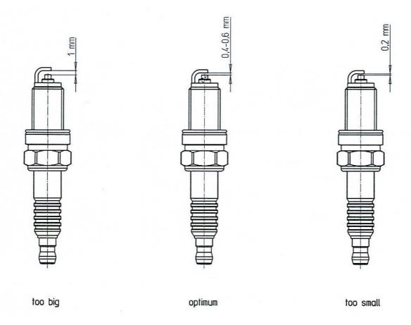
The gap can be set with an inexpensive set of feeler gauges, most auto parts stores or kart shops can supply these for only a few dollars.
