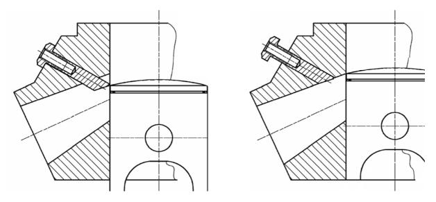
It is clear from the diagram that if the power valve is not fully closed at low (below 7.500) RPM, the exhaust valve do not seal with the piston, resulting in lack of bottom power.
