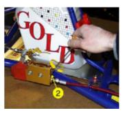
5. Pump 4-5 times <u>very slowly</u> to easier the air come out of the Brake Pump, you will see some bubbles are rising from the pump tank.
